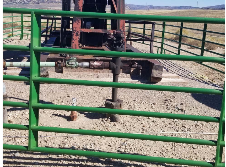
Photo 2. Bradenhead access has been installed.
