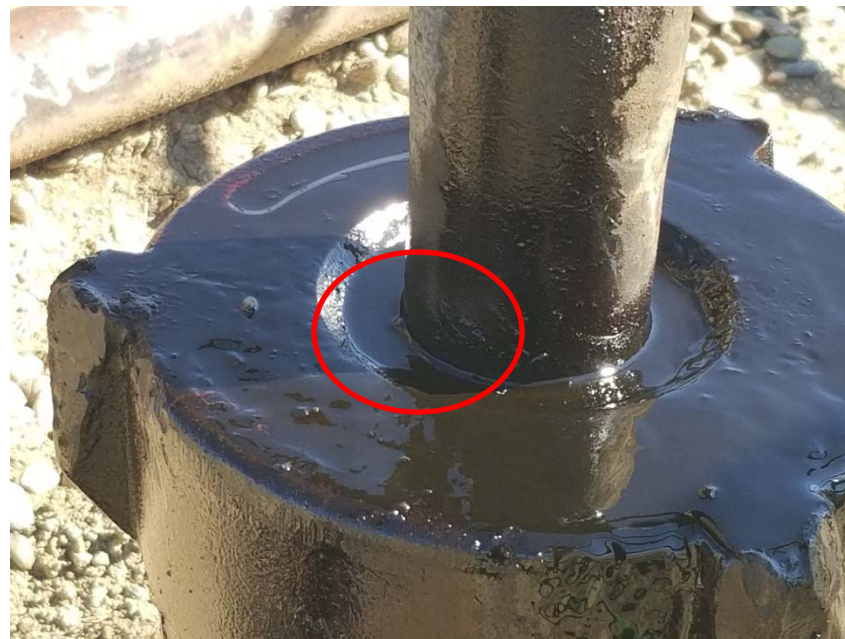
Photo 3. Close up of photo 2, leak occurring at wellhead.
