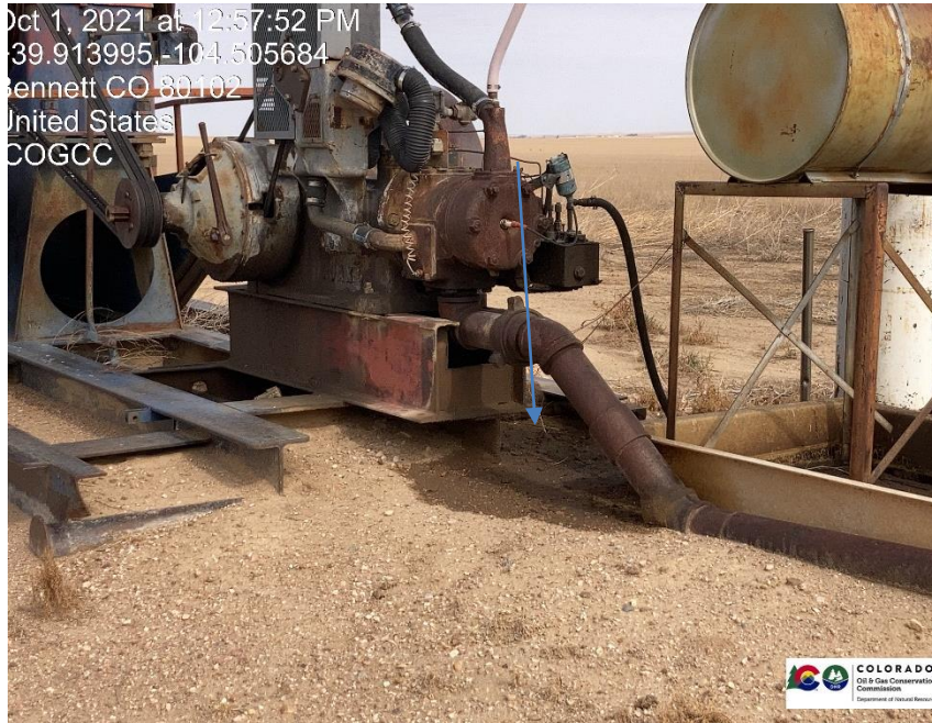
Pic 7 stained soil / mechanical issue with pumping unit motor
