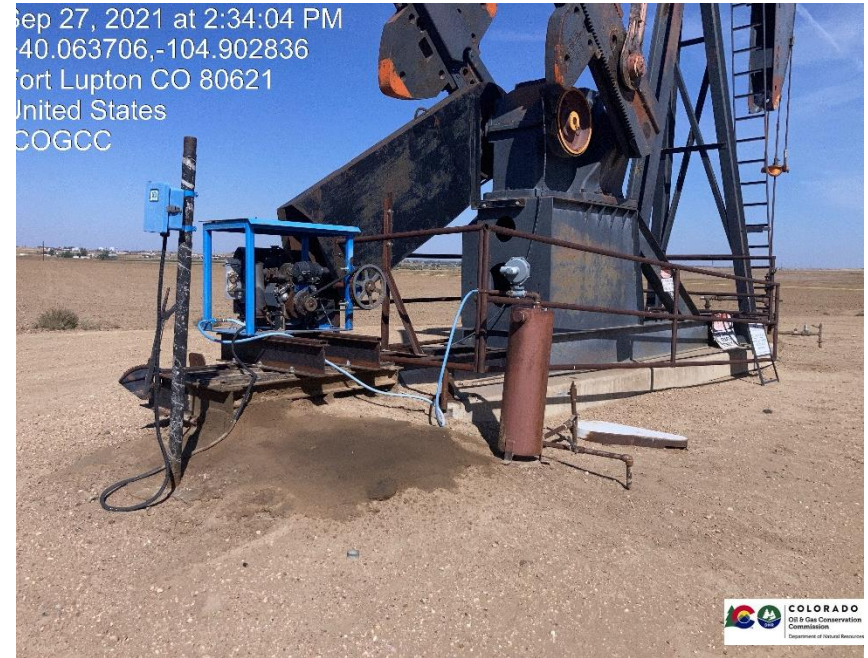
Pic 2 stained soil near pump jack motor/mechanical issue
