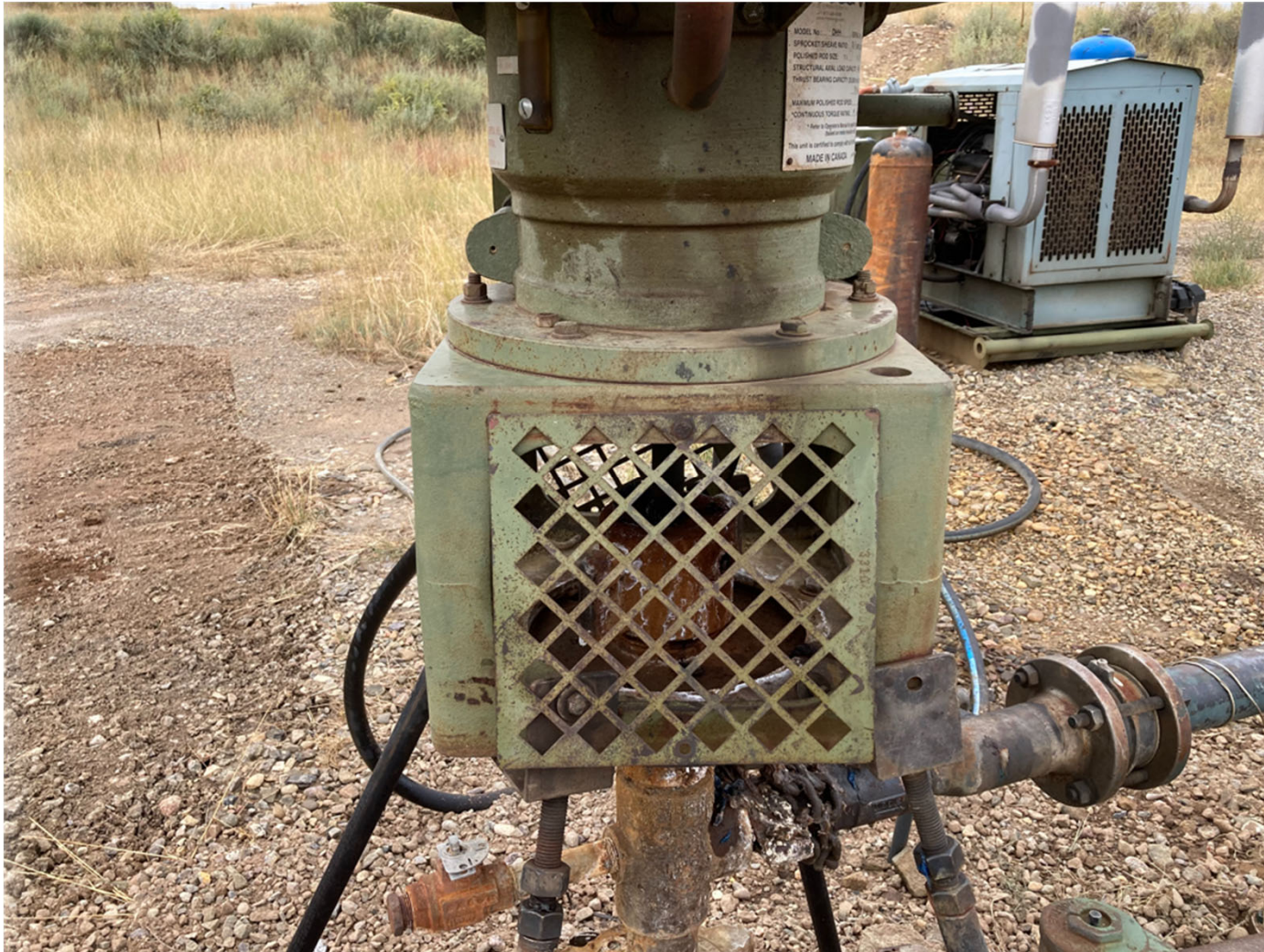
PHOTO 1: THE PACKINGS WERE TIGHTENED TO STOP THE WATER LEAK AT THE WELLHEAD. NO IMPACTS WERE DISCOVERED.
