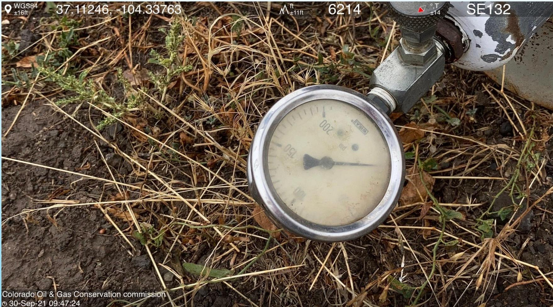
PHOTO 7:BRHD PSI SHOWS 0. I DO NOT BELIEVE THIS GUAGE IS FUNCTIONAL. NEEDLE VALVE IS SHUT IN.
