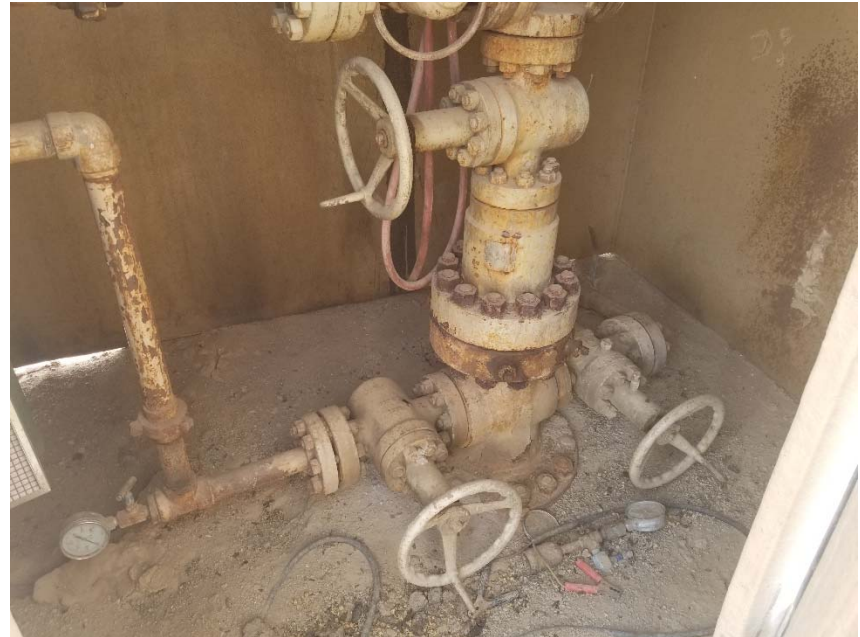
Photo 2. No bradenhead access apparent.
