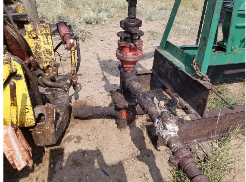
Photo 2. No bradenhead access apparent. Stained soil.
