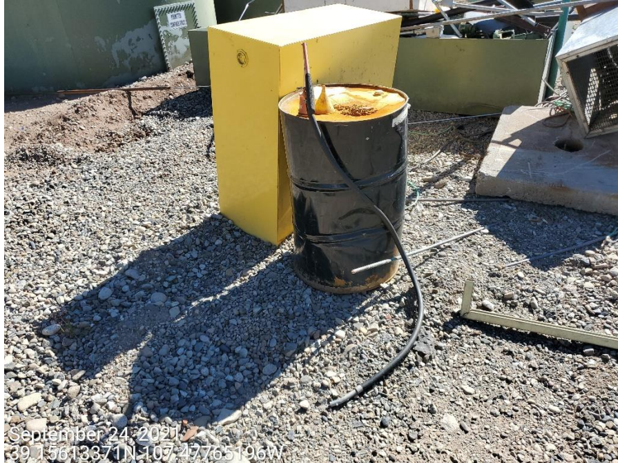
Photo 4: Photo shows example of unused equipment/trash/debris not necessary for production stored on the Location. Photo also shows barrel with inadequate spill prevention or containment BMPs
