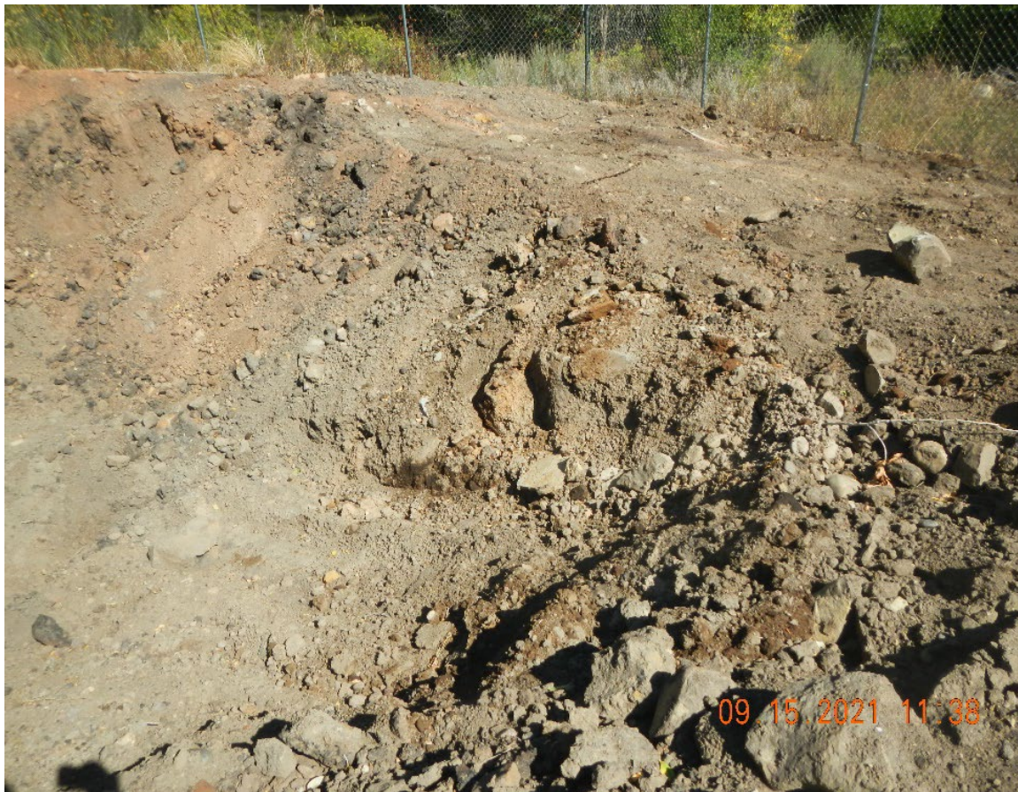
Photo #5 Stained soil observed, soil had strong hydrocarbon odor.
