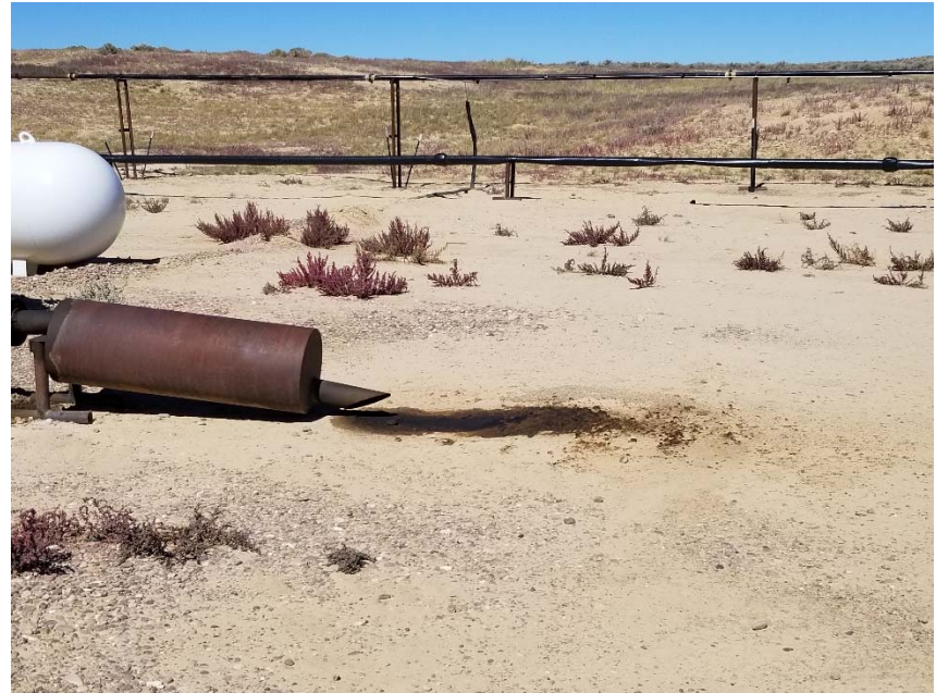
Photo 4. Stained soil at pump jack exhaust.
