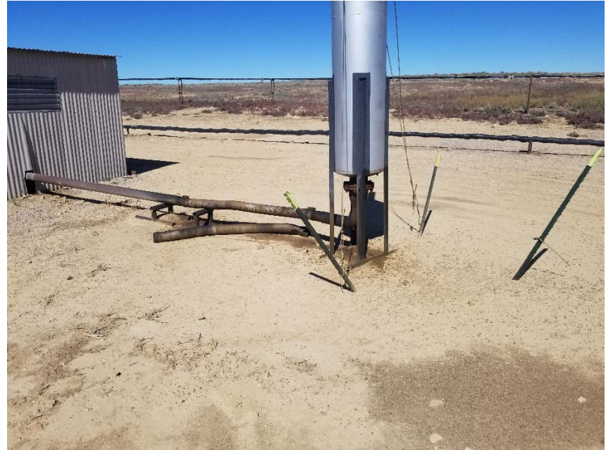
Photo 2. Stained soil at pump jack exhaust line.
