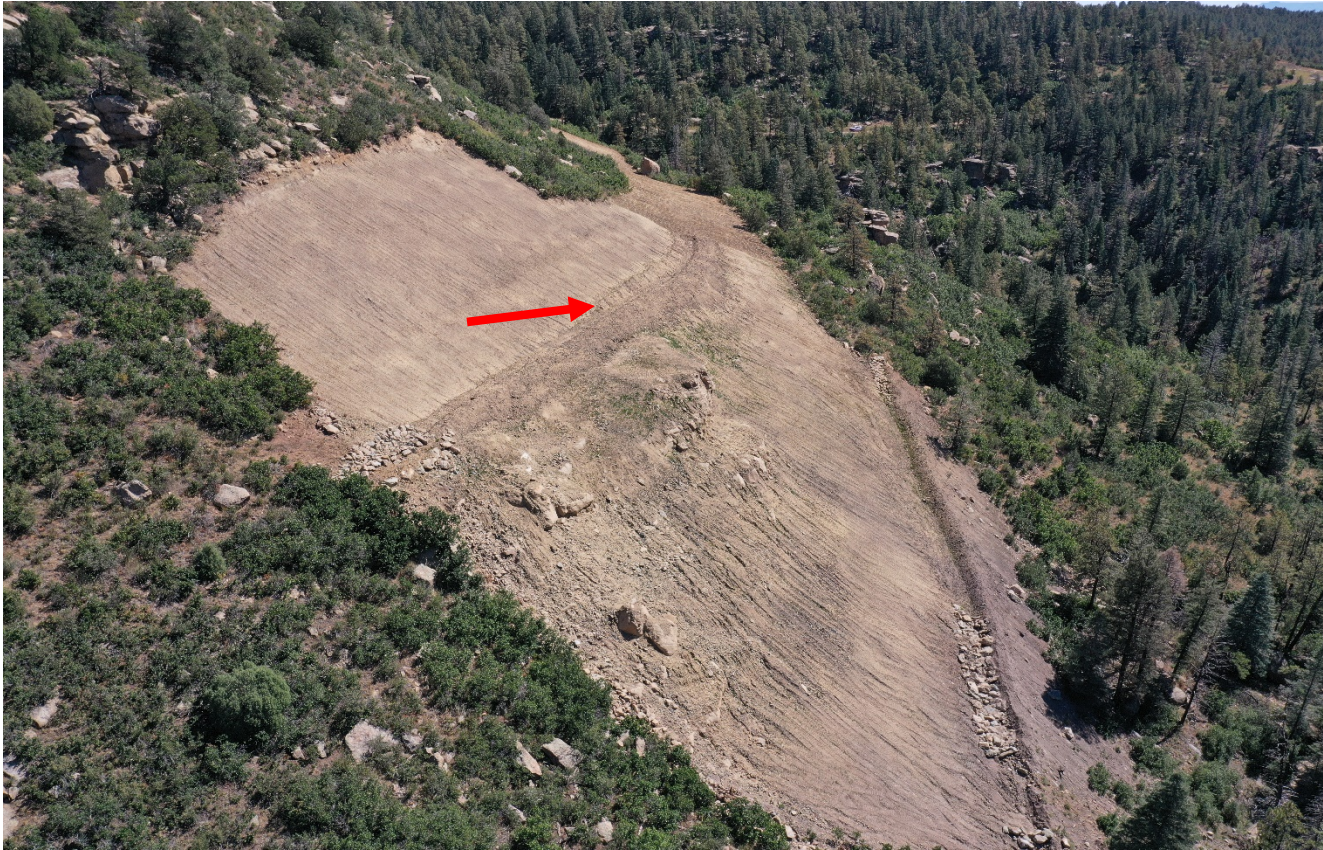
Photo 7. Facing east toward the reclaimed location. A berm is installed at red arrow which appears to be directed east with no stormwater control. This needs to be monitored and may require additional BMP's.
