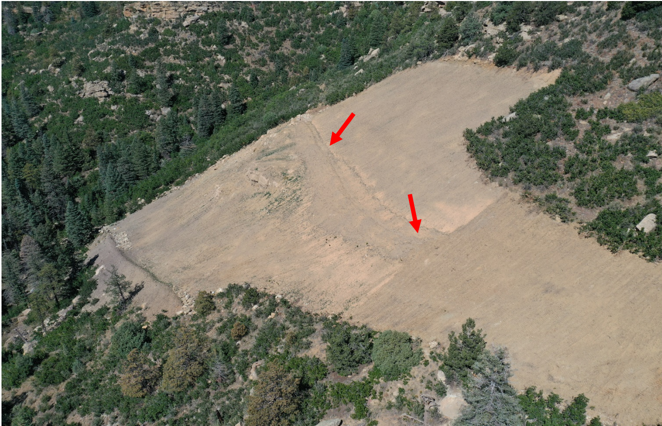
Photo 2. Drone aerial photo facing northwest toward the reclaimed location. A berm is installed at red arrow which appears to be directed east with no stormwater control. This needs to be monitored and may require additional BMP's.
