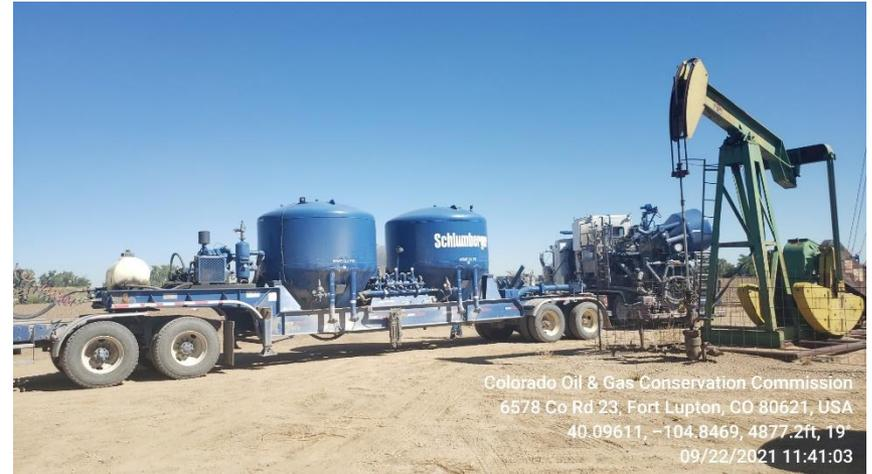
Photo 7 fresh water truck and cement pump truck
