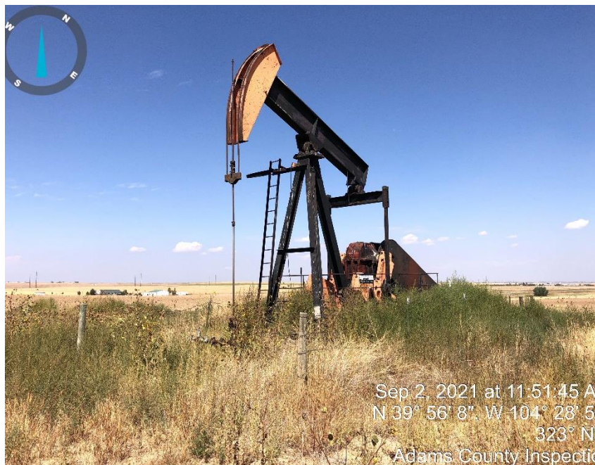
Photo #4 Pump Jack.
