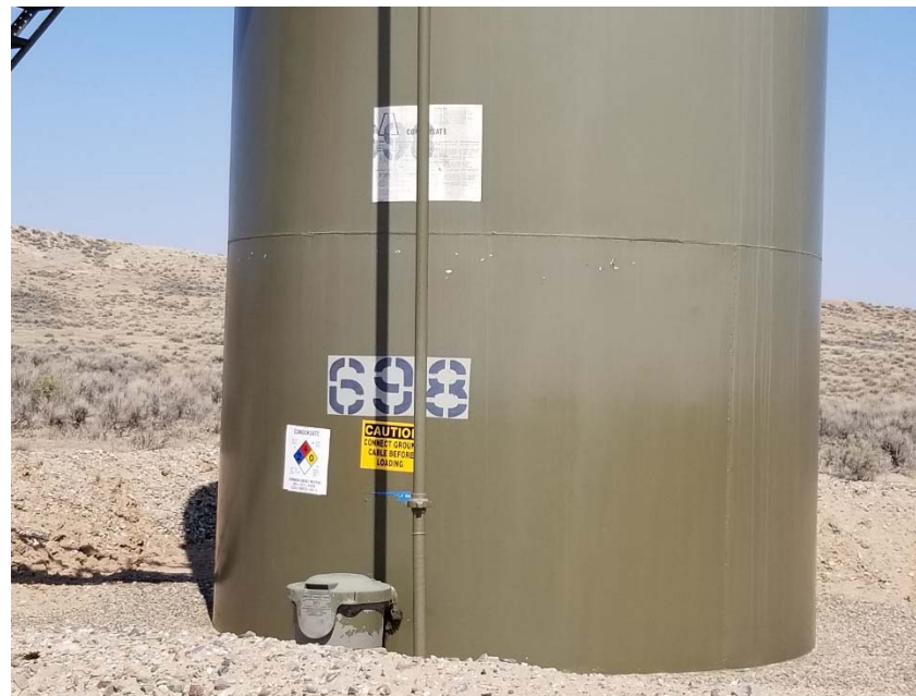
Photo 2. No capacity on condensate tank label.
