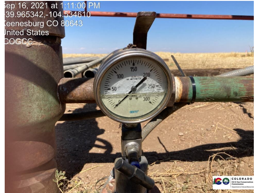
Pic 4 pressure of bradenhead start of bradenhead test
