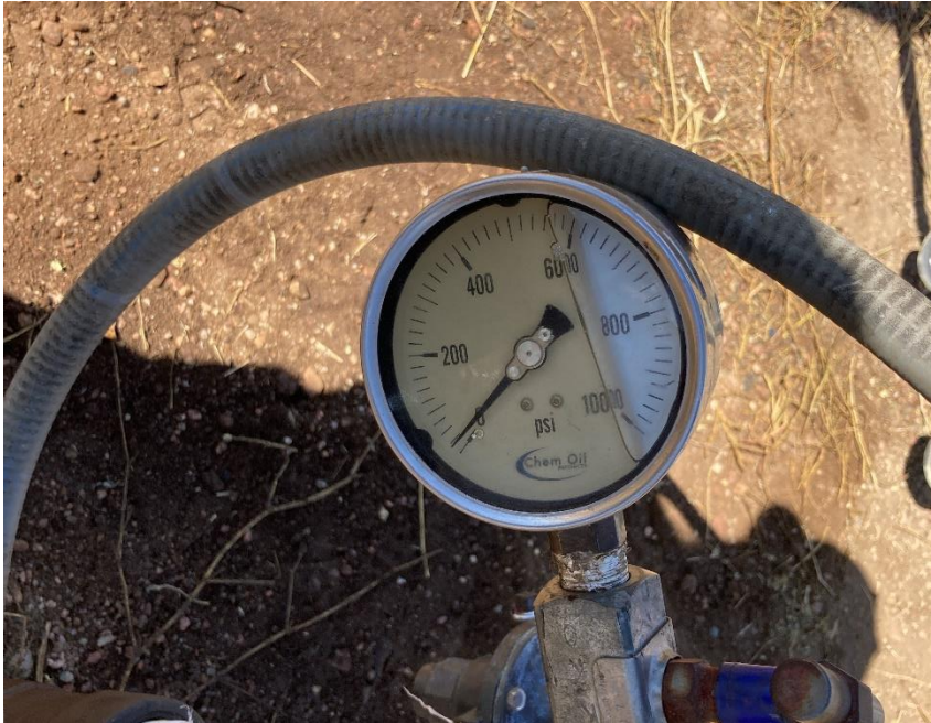
Pic 3 pressure of casing start of bradenhead test
