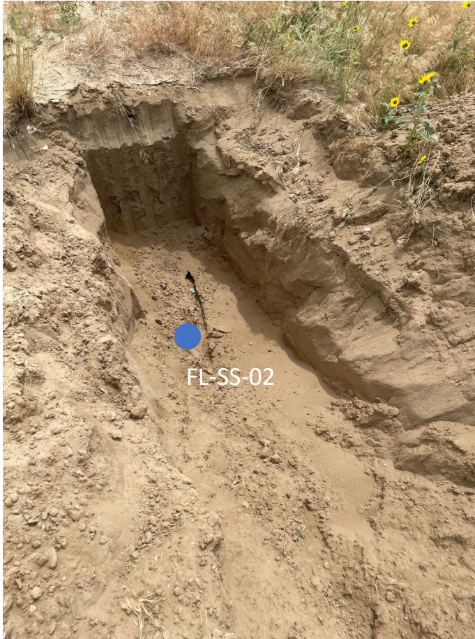
Flowline removal Bellholed/pulled prior to assessment No petroleum hydrocarbon staining or odor observed Screening sample collected: FL-SS-02 @ 3.5' = 0.7 ppm-v
