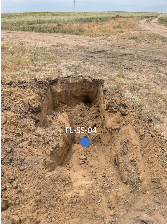
Flowline removal Bellholed/pulled prior to assessment No petroleum hydrocarbon staining or odor observed Screening sample collected: FL-SS-04 @ 3.5' = 2.1 ppm-v
