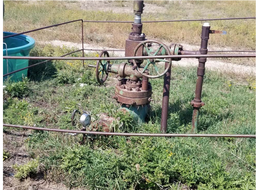
Photo 2. No bradenhead access apparent.
