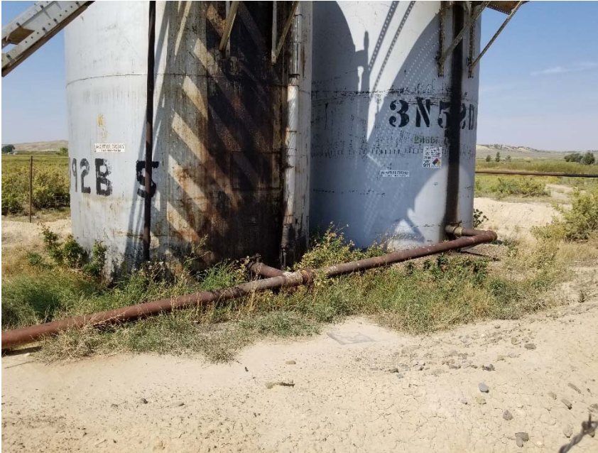
Photo 3. Incomplete label on left hand tank.
