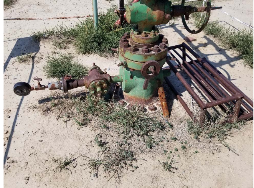
Photo 2. No bradenhead access apparent.
