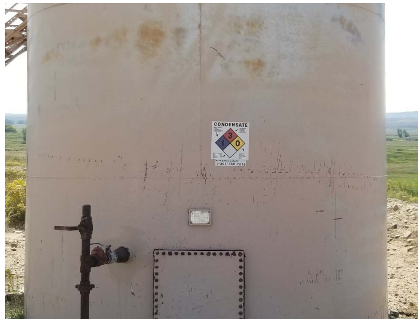
Photo 8. Incomplete tank label.
