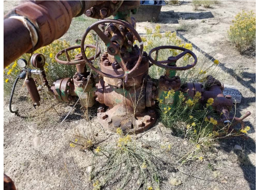
Photo 4. No bradenhead access apparent.
