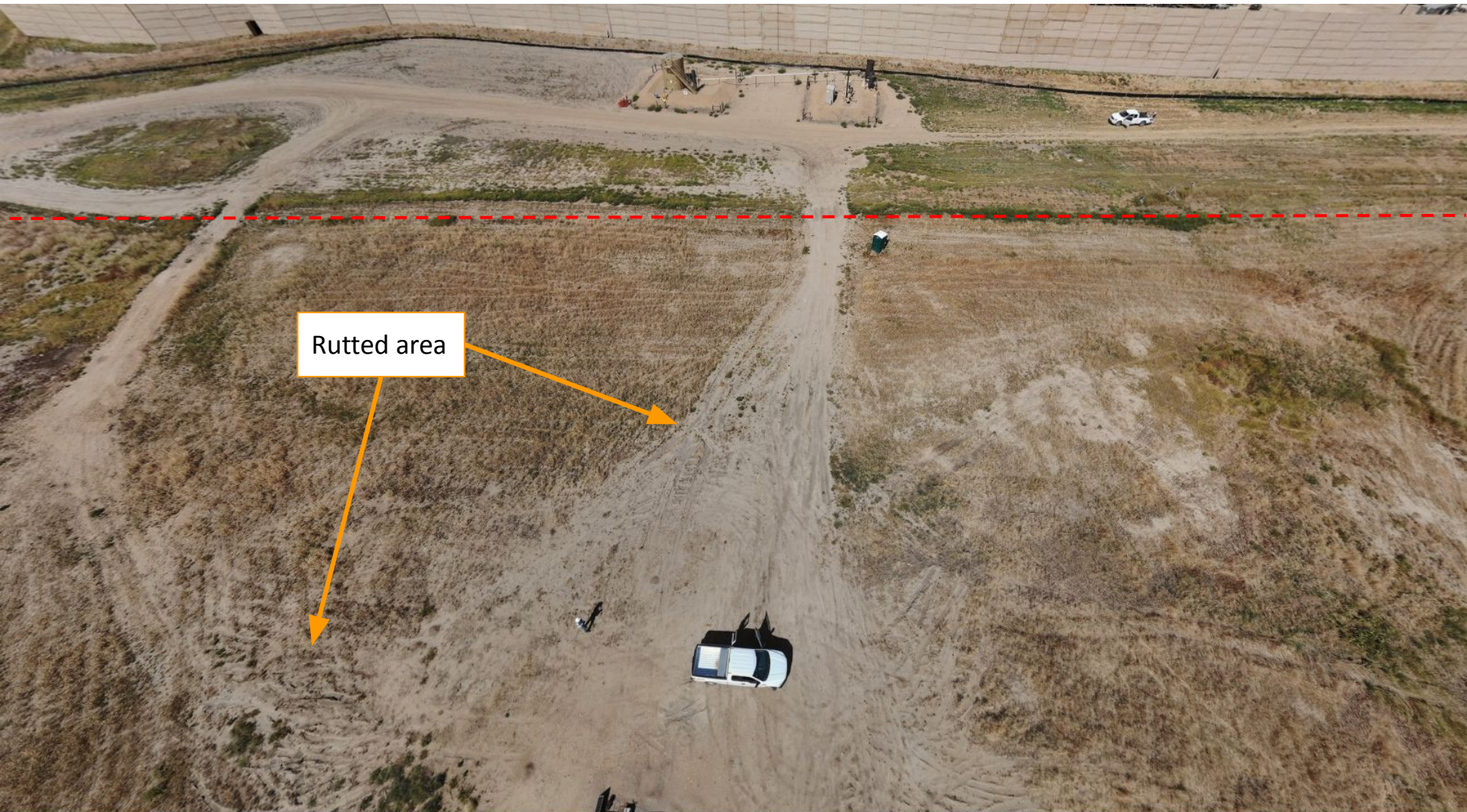
Photo 2. Drone aerial imagery taken from the well location, facing West. Photo illustrates the approximate property line and some of the observed rutted areas. Photo also illustrates unmanaged weeds around the tank battery location- see Photos 9&10.
