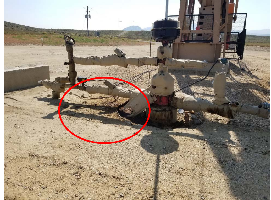
Photo 2. Stained soil at wellhead.
