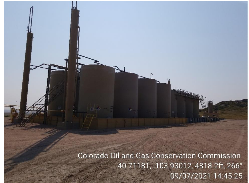
Photo 2 – Tank Battery
