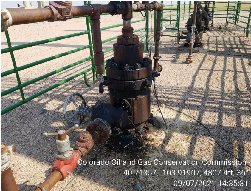
Photo 9 – Stained Soil at 7-36-9-59 Wellhead
