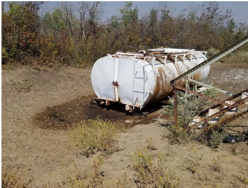
Photo 9. Stained soil at tank.
