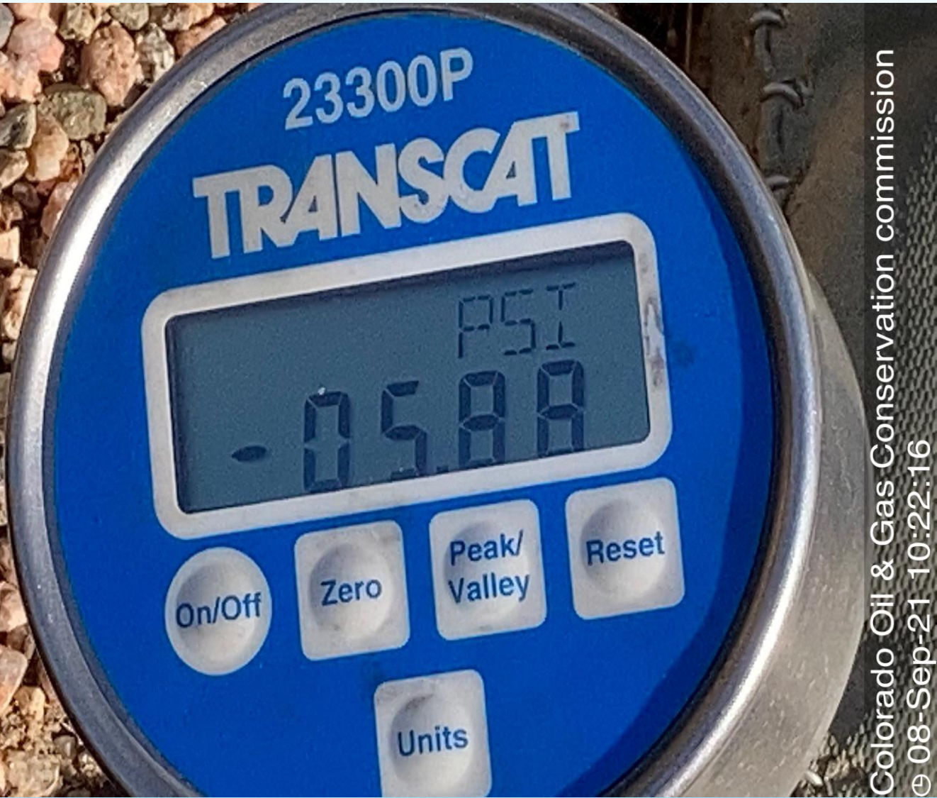
PHOTO 3: TBG/CSG ANNULUS PSI 05.88, PSI EQUILIZED IN 60 SECONDS NO FLUID TO SURFACE
