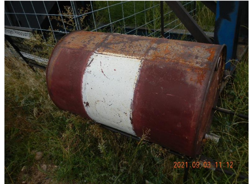
Photo 14: View of disconnected/empty 55 gallon drum on skid mount inside pumping unit fencing.
