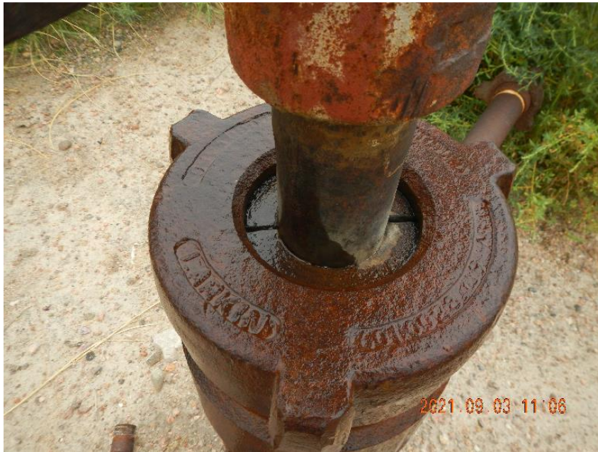
Photo 9: View of packing and cap.
