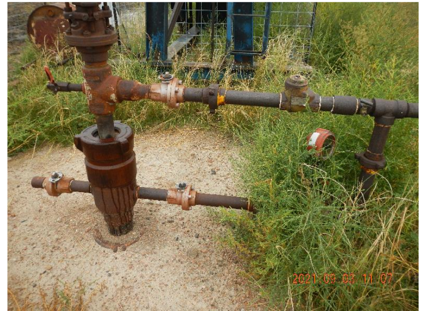
Photo 8: View of wellhead and tree. Well actively venting at packing/cap. Valves were found closed at time of inspection.
