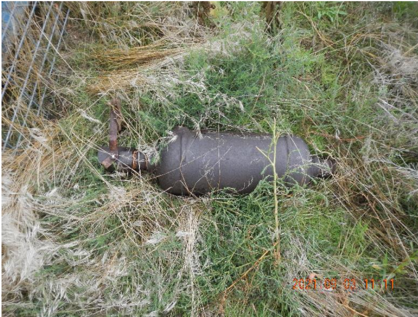
Photo 13: View of disconnected dryer vessel laying inside pumping unit fencing.
