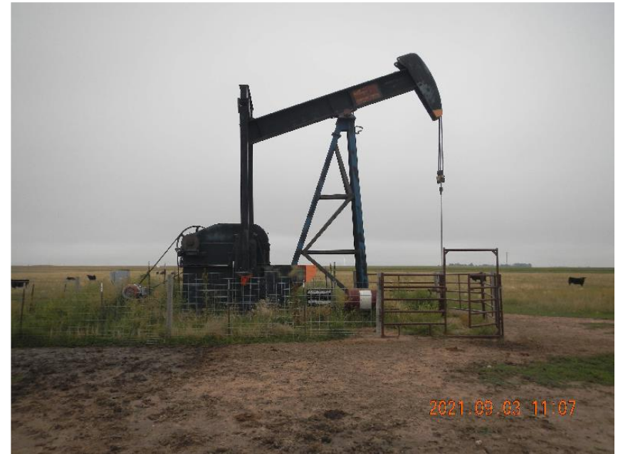
Photo 10: View of pumping unit and vegetation inside the fencing. Polish rod is attached to the bridge.
