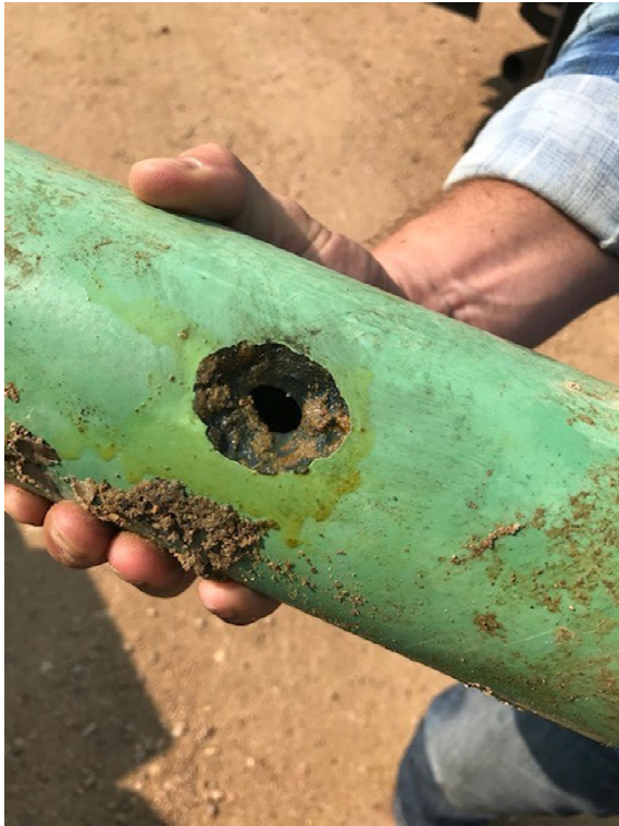
Photos Taken 8/31/2021 – Showing external corrosion hole point of failure.
