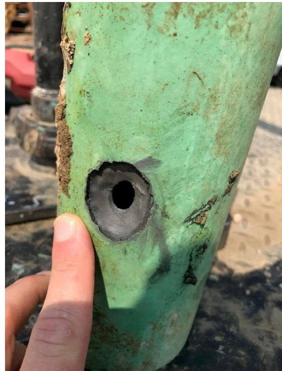
Photos Taken 8/31/2021 – Showing external corrosion hole point of failure.
