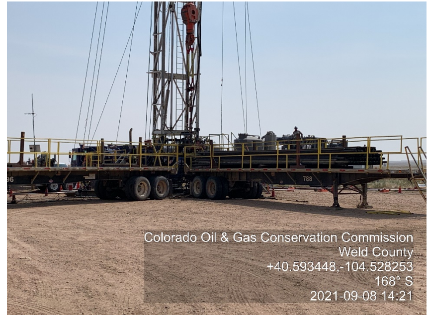
Photo #2 Cummins AB 10-1IJ Wellsite Plugged & Abandoned | PA Plugging Operations: Cementing | Initial Plugs
