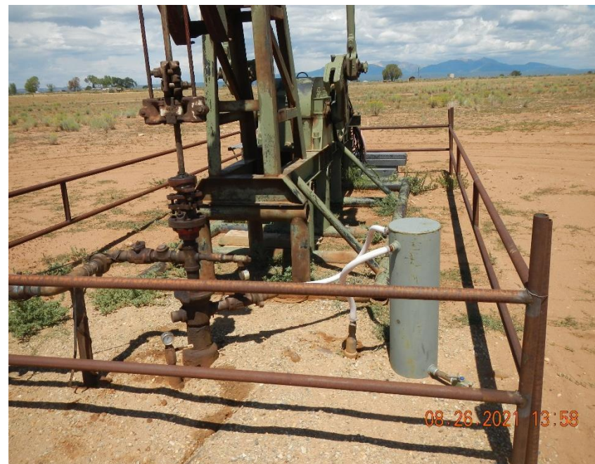
Stained soil around well head.
