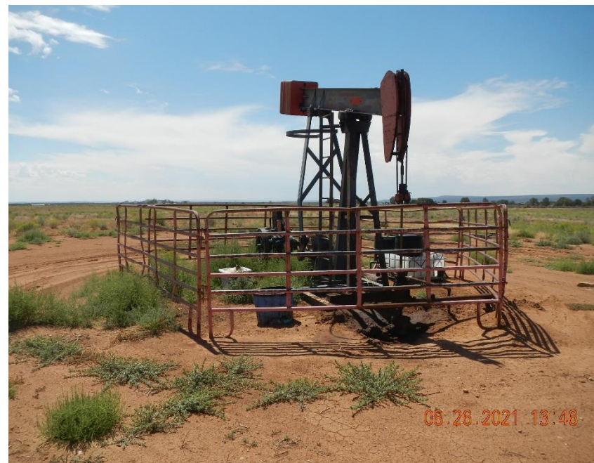
Ted & Hazel #11-1 wellhead and pump jack. Various unused, unlabeled containers stored within fencing.
