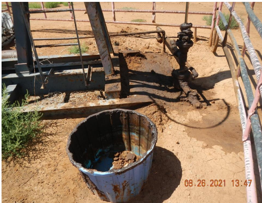
Well head and surrounding area are stained with oil.
