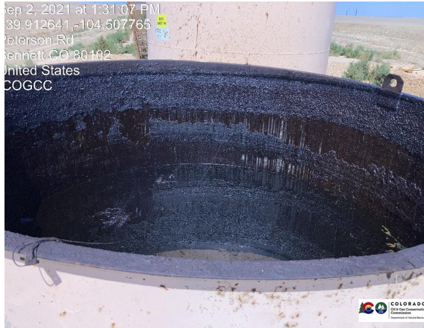
Pic 7 what appears to be dead animals in open top tank, oil present in open top tank, no netting, or content, placard, volume signs.
