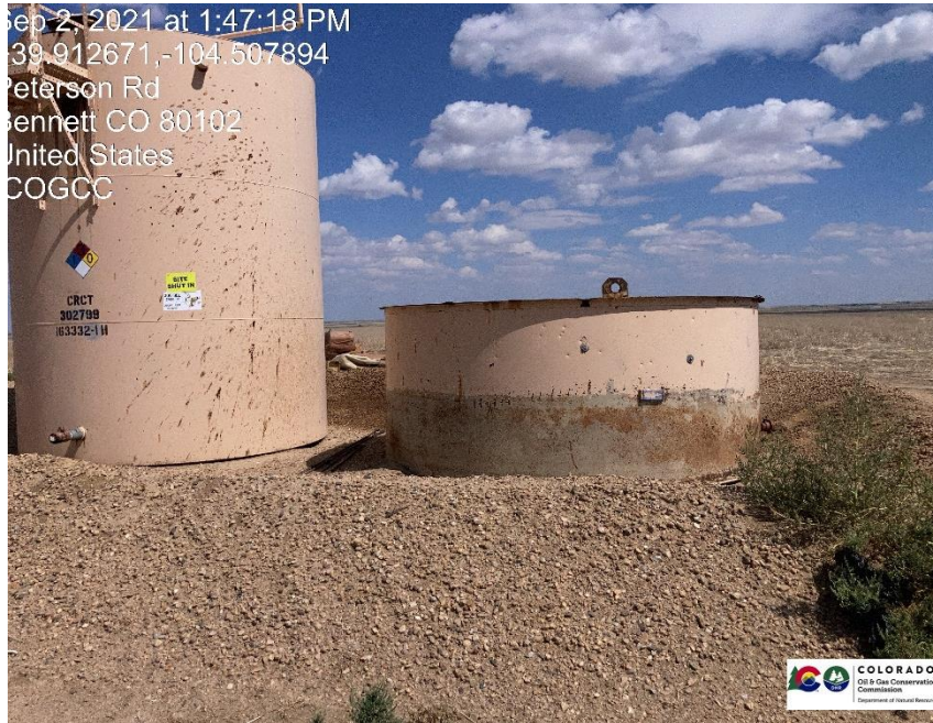
Pic 9 no content, placard, or volume signs on open top tank, with no netting.
