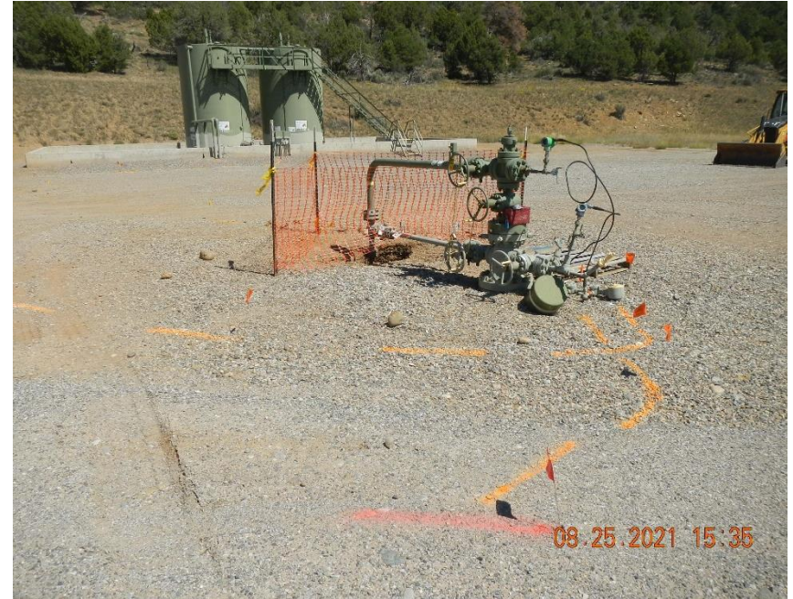
Neleigh 01-07 #1 well head and flow line.
