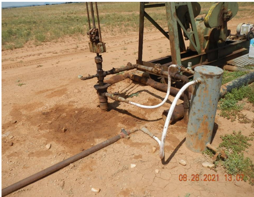
Well head and surrounding soil are stained with oil.
