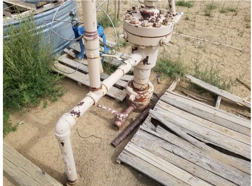
Photo 2. No bradenhead access apparent.
