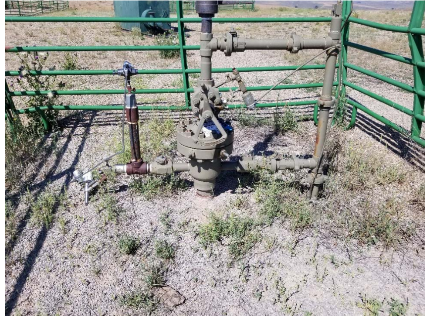
Photo 3. No bradenhead access apparent. Weeds on location.
