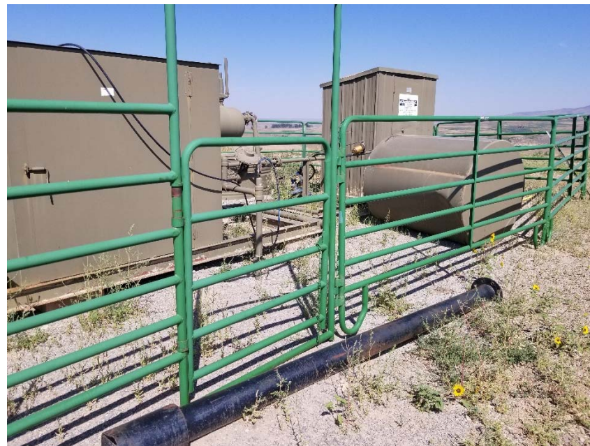
Photo 5. Knocked over methanol tank.
