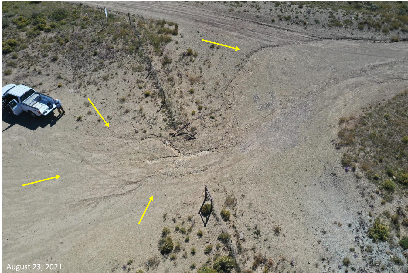
Photo 7: Photo taken with use of a sUAS; aerial photo shows south end of the Location/Location entrance and access road (see photos 4). Photo shows stormwater runoff from the Location has resulted in erosion degradation.
