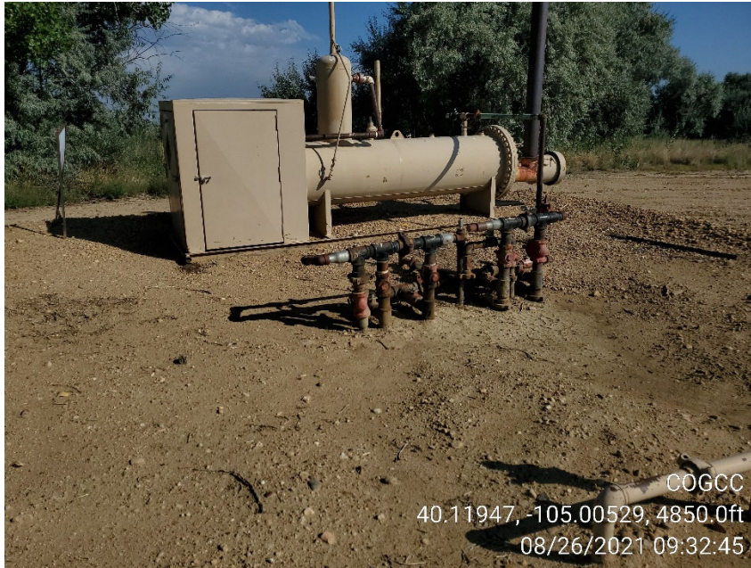
Photo 7 Jillson tank battery header
