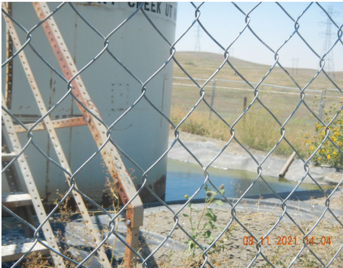
Photo #6 Water inside tank battery.
