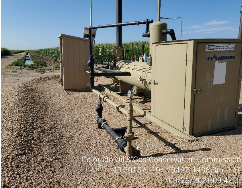
Separator and meter run
