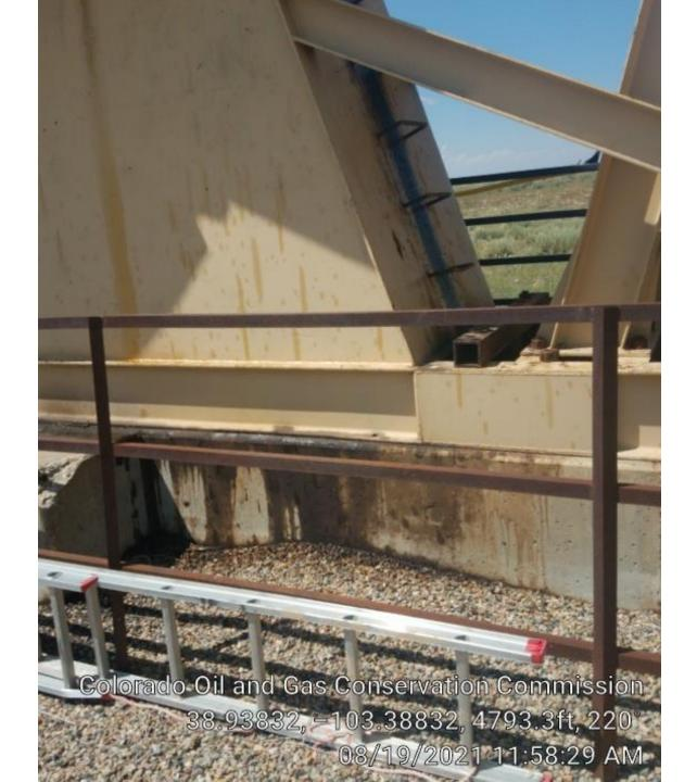
Gear box on pumping unit is leaking and on the ground.
