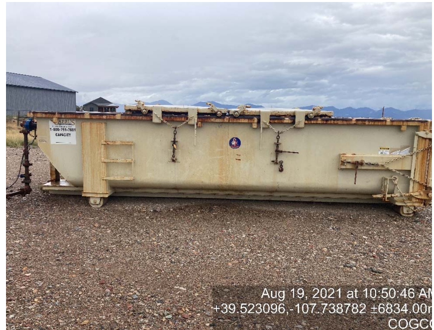
Roll top tank missing signage/lack of containment
