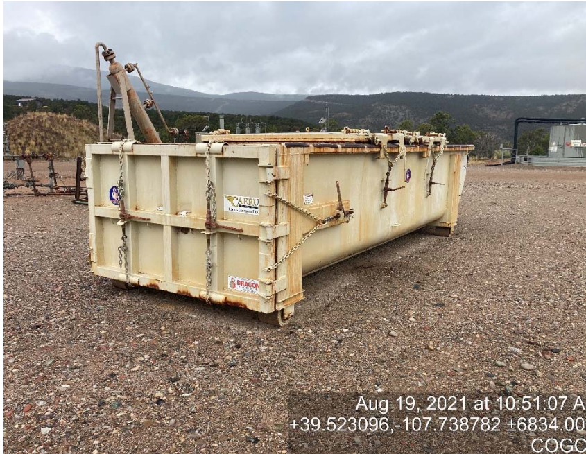
Roll top tank missing signage/lack of containment
