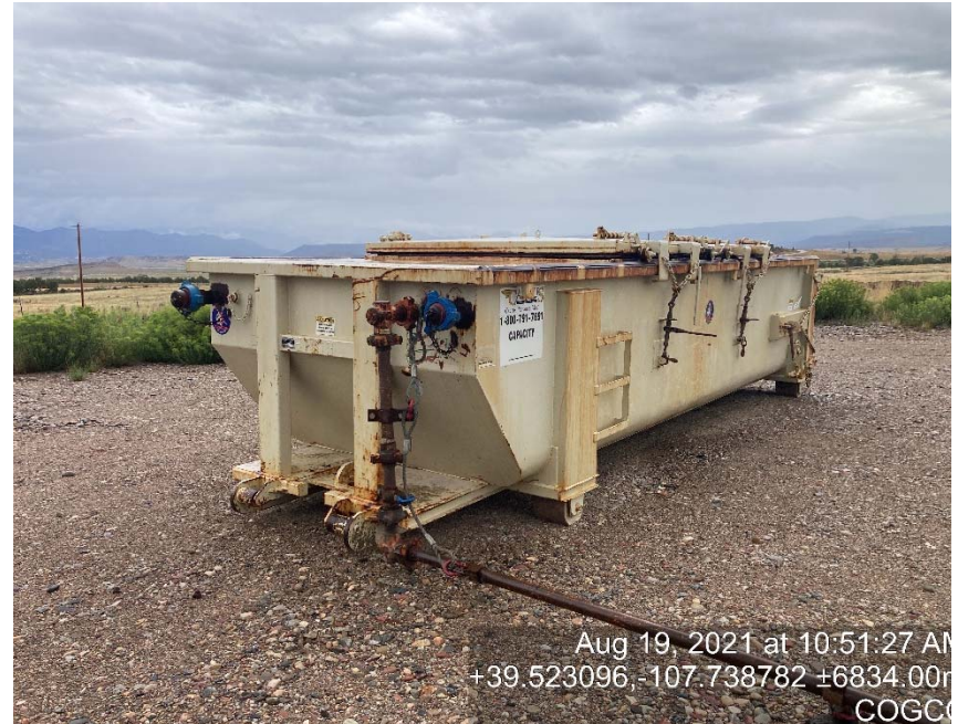
Roll top tank missing signage/lack of containment
