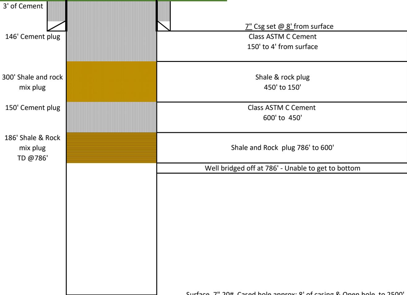
Surface, 7" 20# Cased hole approx: 8' of casing & Open hole to 2500'
