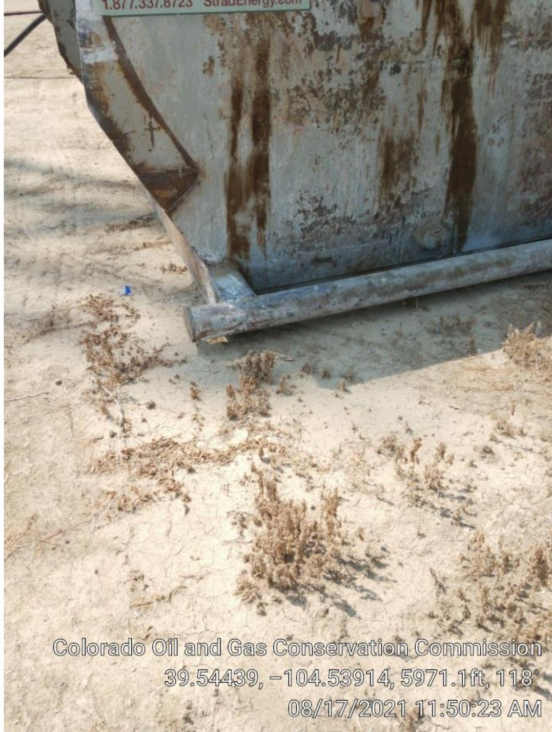
No secondary containment for return tank near drainage on edge of location.
