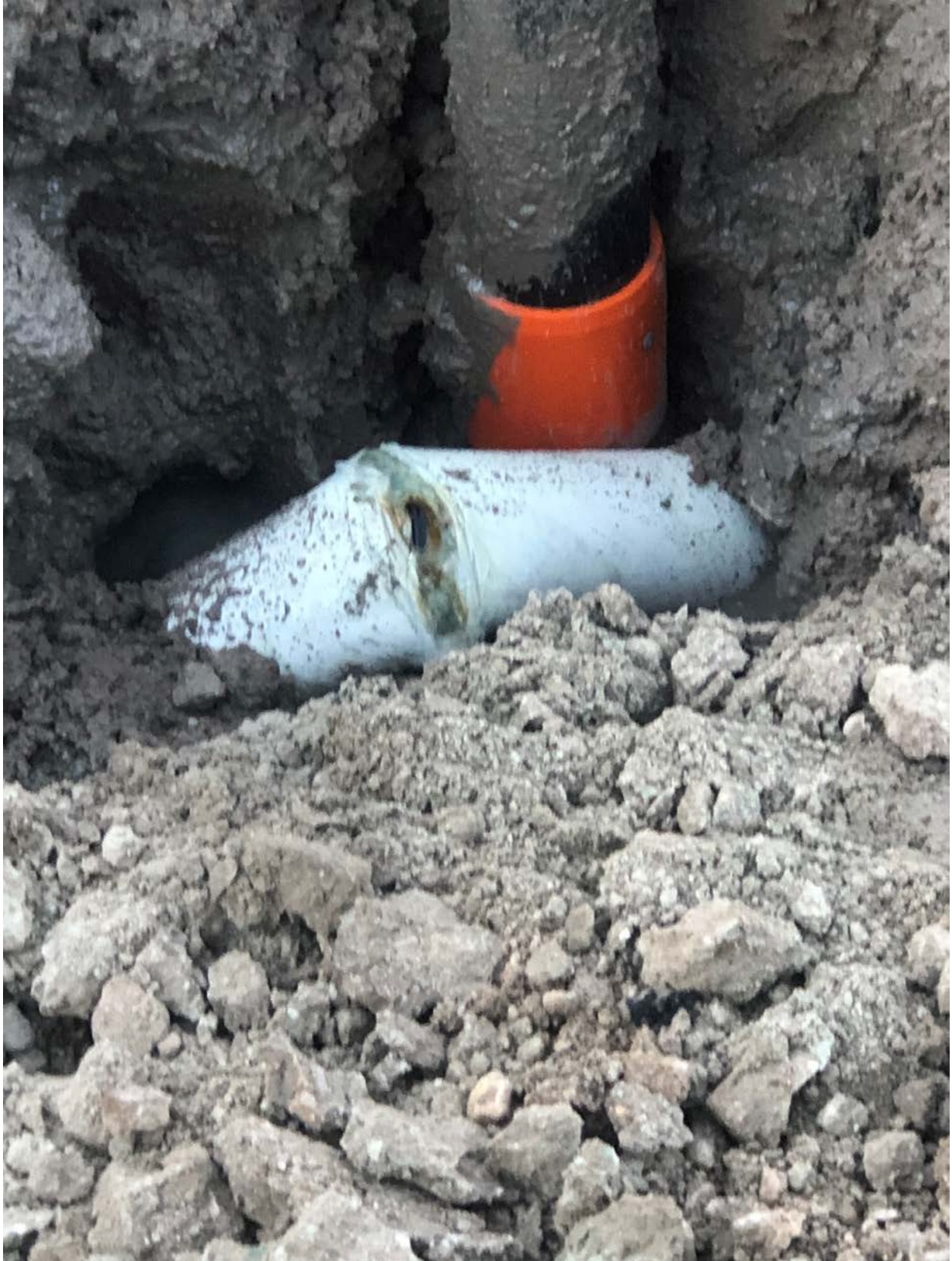
Boomslang 14B initial rupture area
