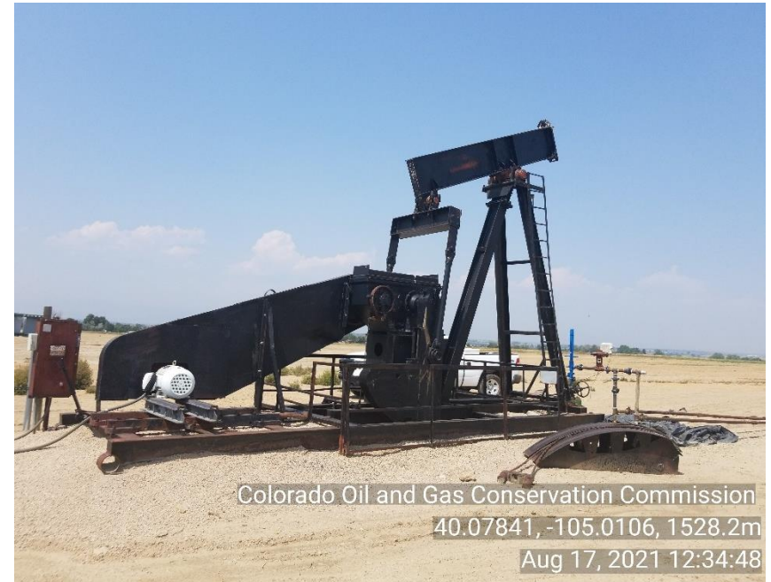
Photo 2 Unused equipment PU and associated equipment.
