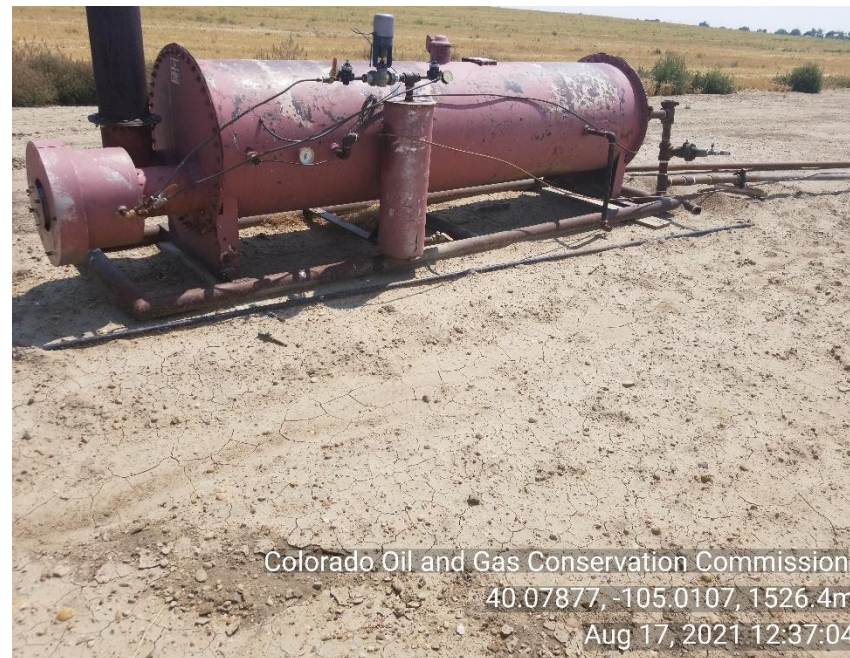
Photo 6 unused equipment: 1" piping and parts around Hoz Separator.
