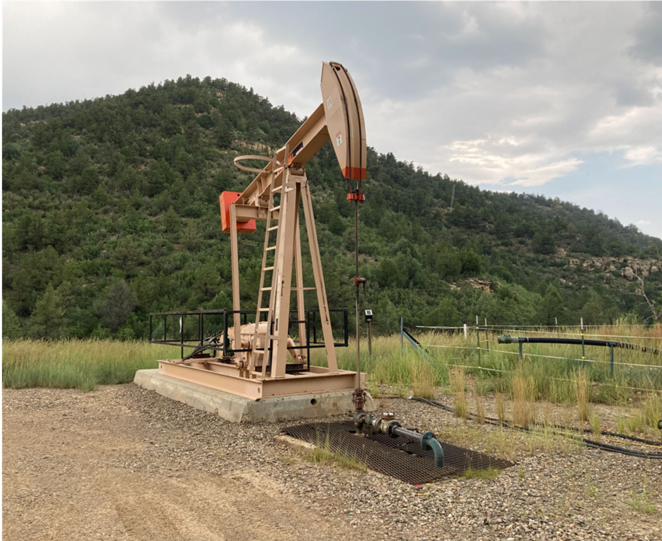
PHOTO 1: THE PC COMPONENTS WERE REMOVED FROM THE LOCATION. THIS WELL WAS CONVERTED TO A JUMPING UNIT. ALL UNUSED EQUIPMENT HAS BEEN REMOVED FROM THE LOCATION.
