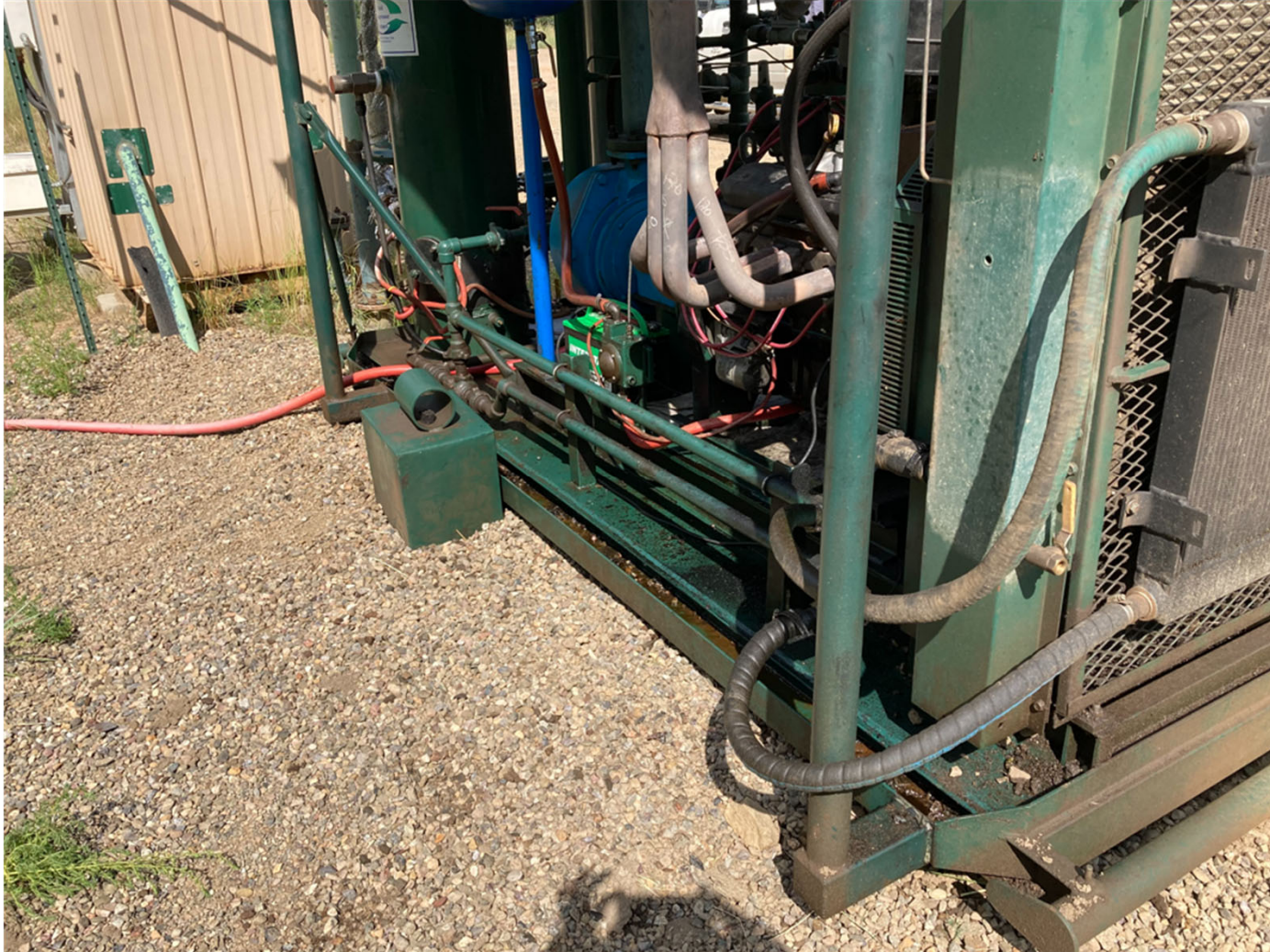
PHOTO 3: THE OIL ACCUMULATION IN THE RESERVOIR OF THE LIQUID RING SKID WAS REMOVED AND THE IMPACTED SOIL NEXT TO THE LIQUID RING COMPRESSOR WAS REMOVED AND PROPERLY DISPOSED IN ACCORDANCE WITH THE OGRIS OPERATING WASTE MANAGEMENT PLAN.
