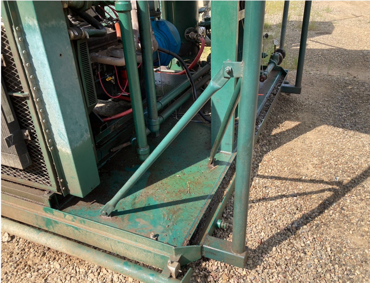
PHOTO 5: ALL VALVES, PIPES AND FITTINGS ARE SECURLY FASTENED. THE OIL ACCUMULATION IN THE RESERVIOR OF THE LIQUID RING SKID WAS REMOVED AND THE IMPACTED SOIL ON THE GROUND WAS CLEANED UP.
