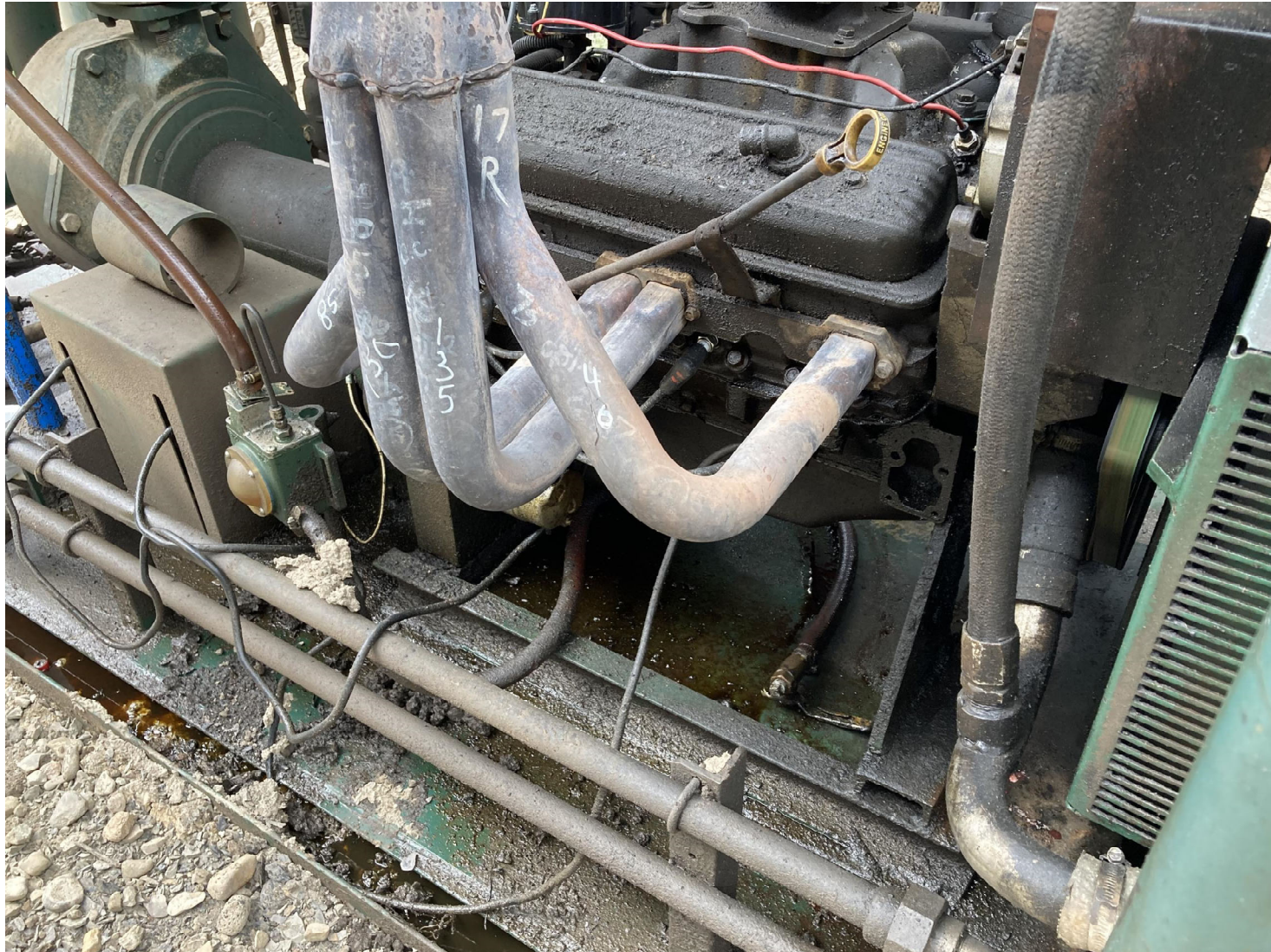
PHOTO 2: THE OIL ACCUMULATION IN THE RESERVIOR OF THE LIQUID RING SKID WAS REMOVED AND THE IMPACTED SOIL ON THE GROUND WAS CLEANED UP.
