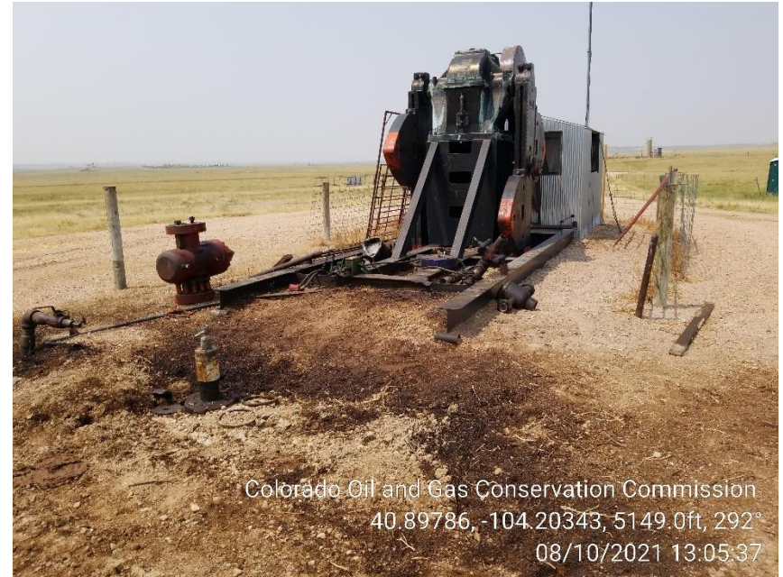
Photo 4 – Wellhead – Stained Soil
