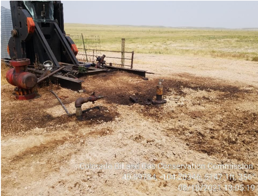
Photo 3 – Wellhead – Stained Soil
